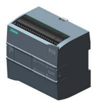
SIMATIC S7-1200, CPU 1214C, compact CPU, AC/DC/relay, onboard I/O: 14 DI 24 V DC; 10 DO relay 2 A; 2 AI 0-10 V DC, Power supply: AC 85-264 V AC at 47-63 Hz, Program/data memory 100 KB
