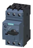
Circuit breaker size S00 for motor protection, CLASS 10 A-release 0.45...0.63 A N-release 8.2 A screw terminal Standard switching capacity
